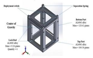
Figure 1: CubeSat Structure
