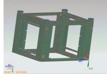
Figure 4: Fix Support in software analysis
