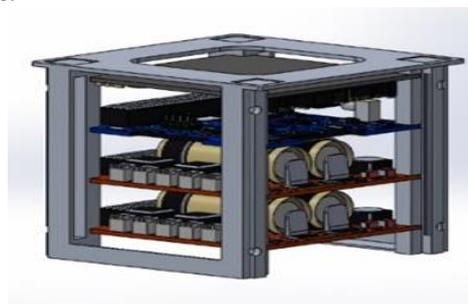
Figure 3: Slotted rack and dummy payloads
