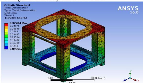
Figure 5(a). Total deformation
