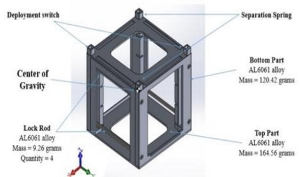
Figure 1: CubeSat Structure
