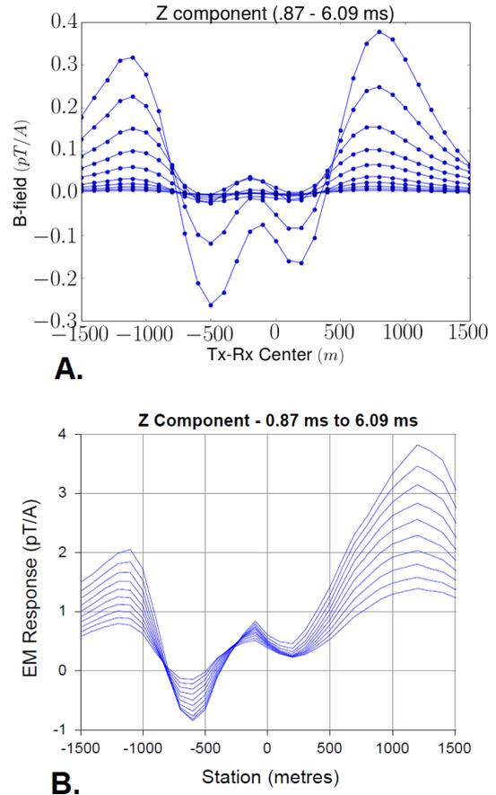
**Figure 4.** Secondary B-field vs distance response at mid-times for one version of the cross-section model (A) and the corresponding ARC SQUIDTEM data (B).
