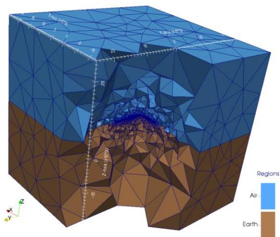
**Figure 1.** Cutaway of a 3D unstructured tetrahedral mesh. The air and earth are colored in light blue and tan respectively with edges of tetrahedra in dark blue. Mesh volume is 50 km<sup>3</sup>.
