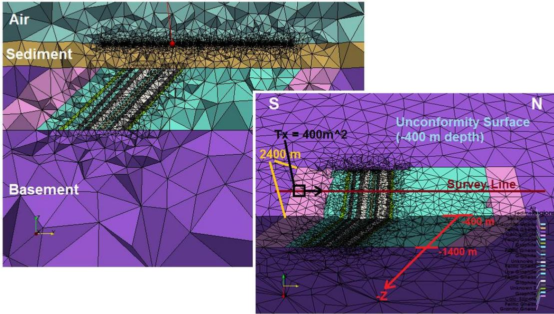
**Figure 3.** At left is a slice along the x-axis of a version of the cross-section model where the graphitic conductor package has a 1 km depth extent, at right is a 2D cutaway of a 3D view of the mesh showing both the strike length and depth extent of the package.
