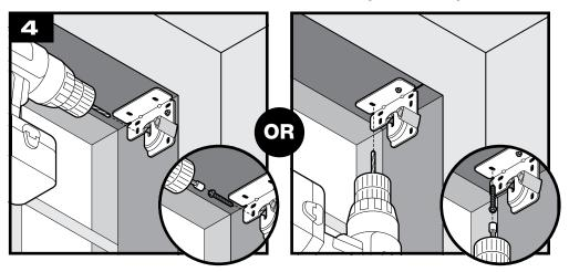
**SIDE MOUNT:** Drill second 3/32" pilot hole. If necessary, use wall anchor (not included). Secure brackets with second screw using 1/4" driver.
