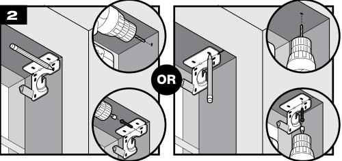
**SIDE MOUNT:** Mark bottom of slotted front hole on side of bracket. Drill 3/32" pilot hole on mark. If necessary, use wall anchor (not included). Secure brackets with one screw using 1/4" driver.
