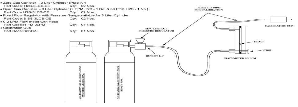
The calibrated range for fixed detectors shall be: a. 0 to 100 PPM - hydrogen sulfide in air (10 ppm & 15/20 ppm) b. 0 to 100% LEL - combustible gas in air. (20% LEL & 60% LEL)
