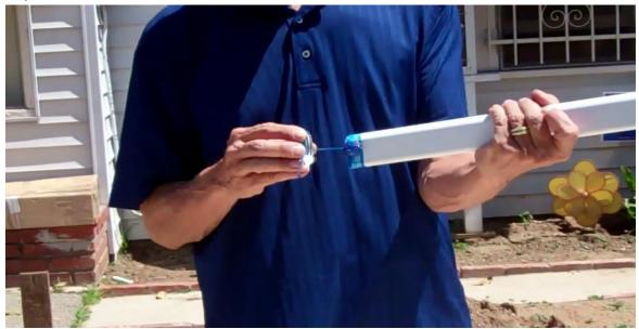
**10.** After you put the glue on the top and sides of the coupler (see below) and the AquaJet you need to push the AquaJet into the coupler and hold it for 5 seconds so it does not slide off.
