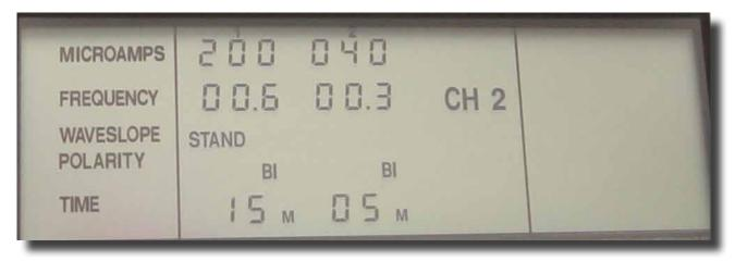
Every setting you can make is at the first level and is visible at all times. Simply select the parameter to change and make the change using the numerical keypad. This can even be done in real time as a treatment is being administered. Each channel has it's own independent timer for treating multiple areas or patients at the same time. You can also use the probe electrodes, which operate off channel 1, and channel 2 at the same time.
