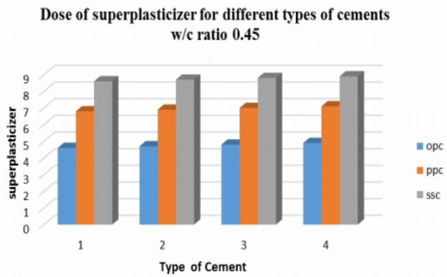
Fig.2: Dose of superplasticizer for different types of cements
