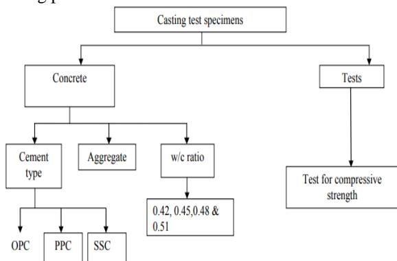
Fig.1: Experiment details for compressive strength
