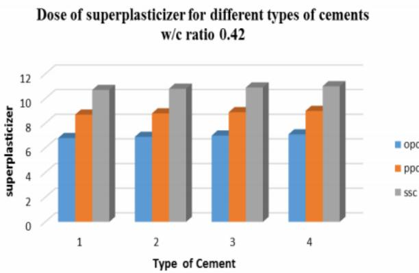
Fig.1: Dose of super plasticizer for different types of cements
