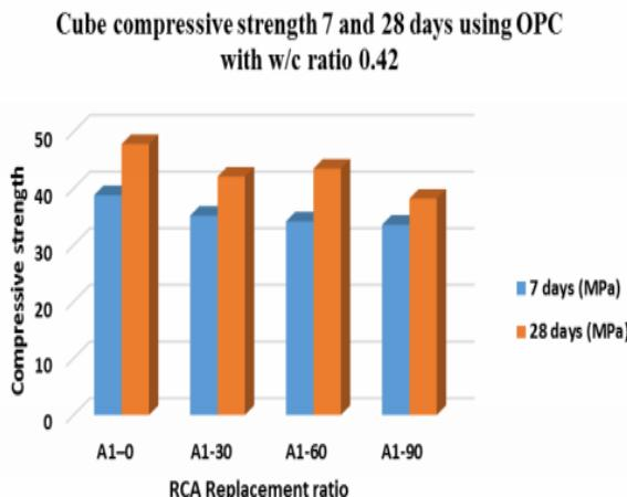
Fig.5: Cube compressive strength 7 and 28 days using OPC with w/c ratio 0.42
