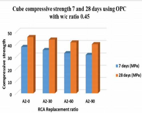
Fig.6: Cube compressive strength 7 and 28 days using OPC with w/c ratio 0.45
