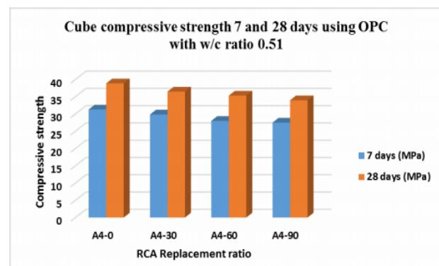
Fig.8: Cube compressive strength 7 and 28 days using OPC with w/c ratio 0.51
