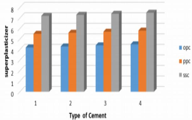
Fig.3: Dose of super plasticizer for different types of cements
