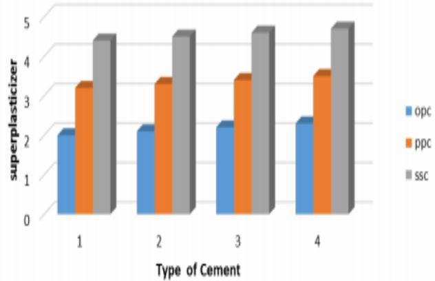
Fig.4: Dose of super plasticizer for different types of cements
