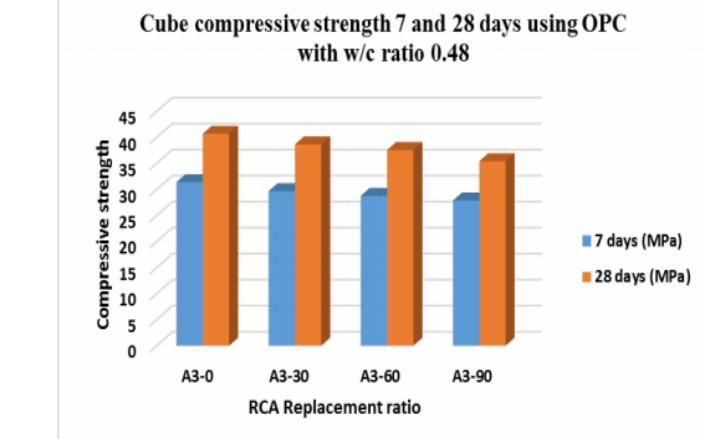
Fig.7: Cube compressive strength 7 and 28 days using OPC with w/c ratio 0.48
