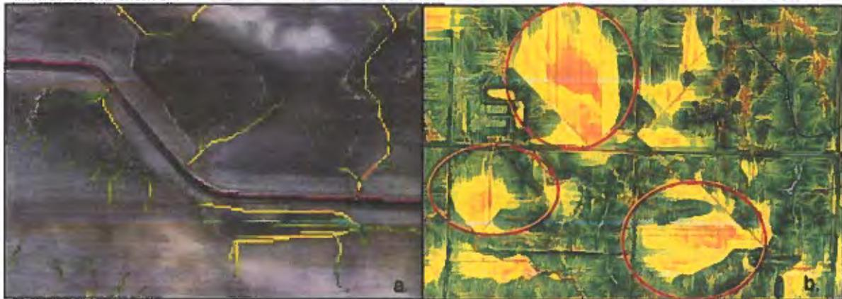
Figure 5. (a) SPI calculation illustrating flow intensity across a field and draining to a nearby ditch. (b) CTI calculation identifying flow accumulation in depressional areas where ponding is expected to occur.
