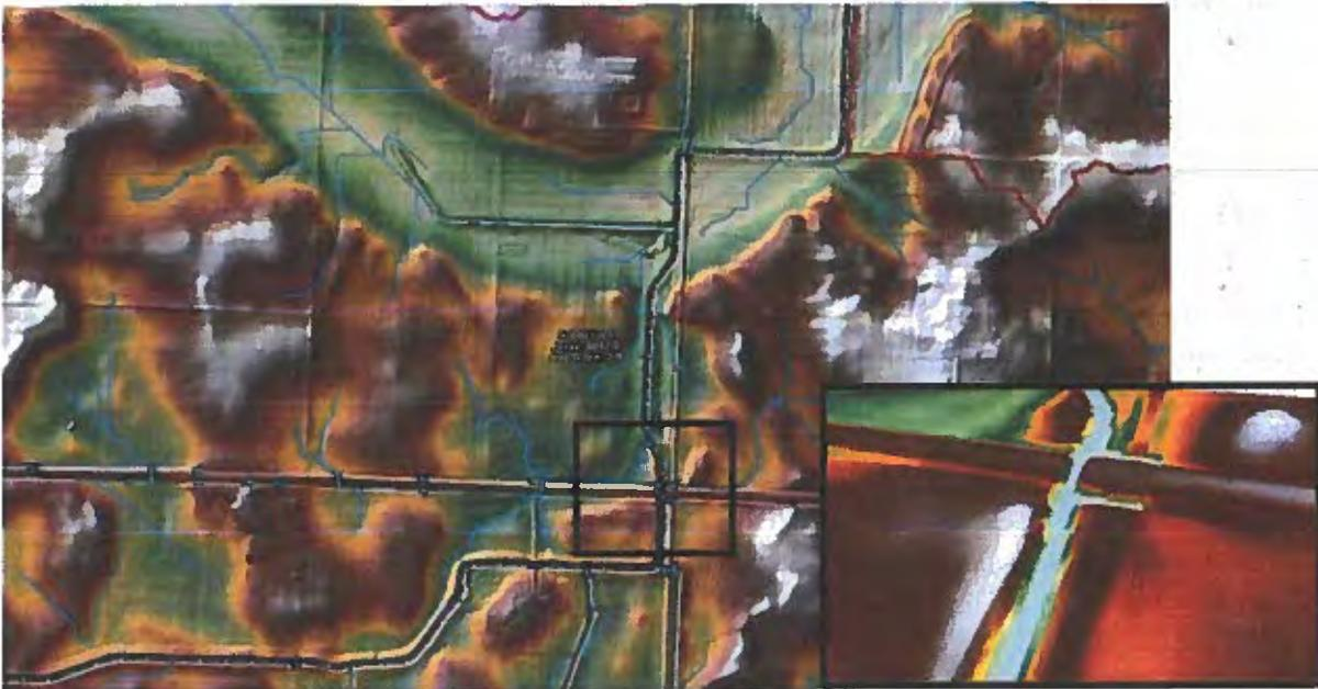
Figure 3. Flow path adjusted to model surface water flow through water conveyance infrastructure.
