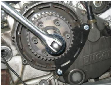
**CAUTION: The nut is very tight and will take much effort to loosen with a breaker bar. Personal injury or equipment damage is possible**
