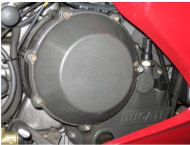
Remove the 5mm Allen bolts securing the cover to the case. After the cover is removed, inspect the gasket for wear and defects. The gasket pictured was installed incorrectly was subsequently worn away by the rotating clutch,
