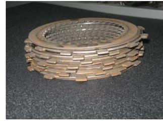
Inspect the condition of the tangs on the clutch basket. If the ridges are very noticeable, these will contribute to premature wear of new clutch plates: the bigger the gap between plates and basket means more wear on the clutch plate tangs.
