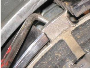
Using the picks provided, remove the friction plates and the spacer plates. Keep the plates in order in case the plates are used on reassembly.
