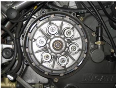
Remove the 4mm Allen bolts securing the pressure plate; place the springs and hardware in a safe place for reinstallation.
