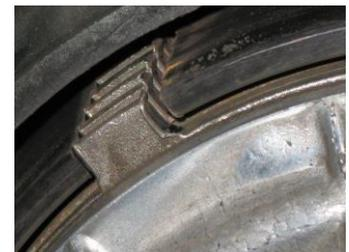
Carefully remove the pressure plate: the clutch pushrod has a tendency to come out with the pressure plate. Try to leave it in place if possible. Inspect the pressure plate for cracks/damage/wear. Inspect the springs and retaining bolts. Replace if necessary.
