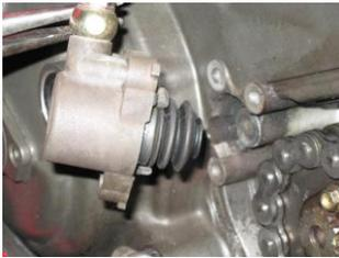
Remove and inspect the condition of the slave cylinder and the associated seal.
