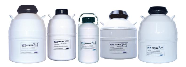
The Doble Series cryogenic liquid dewars are the first units to be designed for both vapor shipment and liquid storage. A unique absorbent layer in the base of the storage tanks of both series enables them to be charged with nitrogen and employed as dry shippers with hold times of up to 30 days. Once at the final destination, the tanks can be filled with liquid and used for long term storage, therefore avoiding the need for return shipments.
