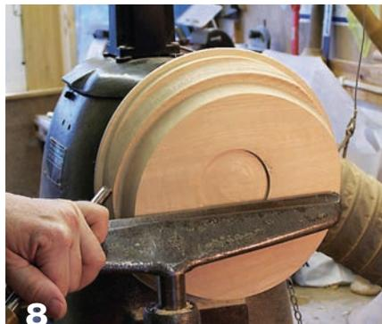
**8** With the lathe stopped, it is easy to see how the offset mounting affects the cutting of the platter's rim.
