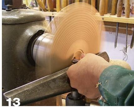
13 Start to hollow out the platter, which is mounted on the newly cut recess.
