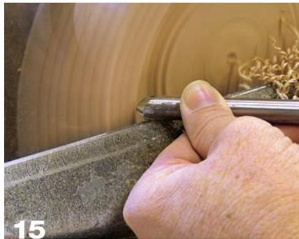
15 To begin hollowing, hold the flute at 3 o'clock. The bevel will head straight into the spinning beads. Once safely past this point, rotate the tool to a more open position.
