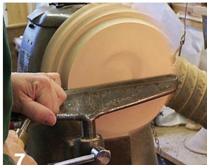
**7** Cut away the bulk of the off-center rim. Work from the outside in stages, pivoting the gouge into the blurred spinning wood.
