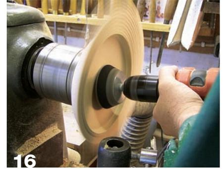
16 With a 3"-diameter soft disc, sand the interior of the bowl.
