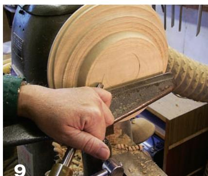
**9** Cut away the first recess and make a flat bottom. Then mark for the new recess that will be centered on the new axis.
