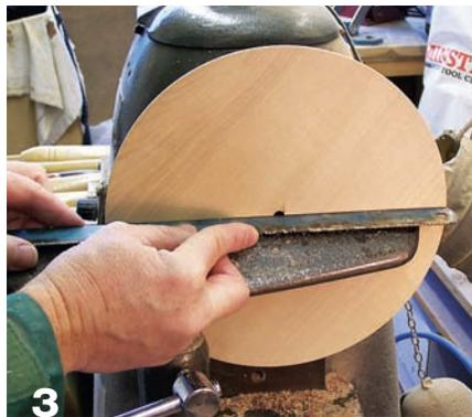
**3** Turn a flat top to the platter and check with a straightedge.
