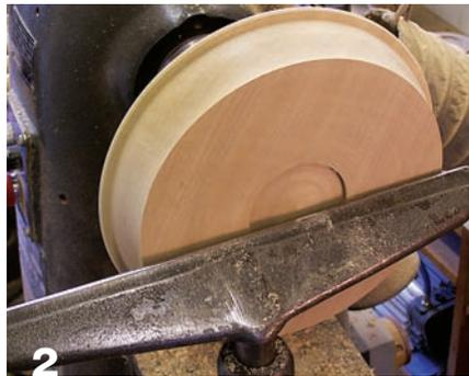
**2** Flatten the bottom, make a recess for the chuck, and establish a rounded edge.
