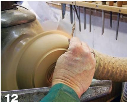
12 Sand what you can on the bottom now, as you won't be able to come back to it later. Sand the overhanging flange of the rim with the lathe off.
