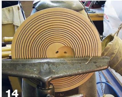
14 Although it looks odd, the hole on the right is the new center of the platter.
