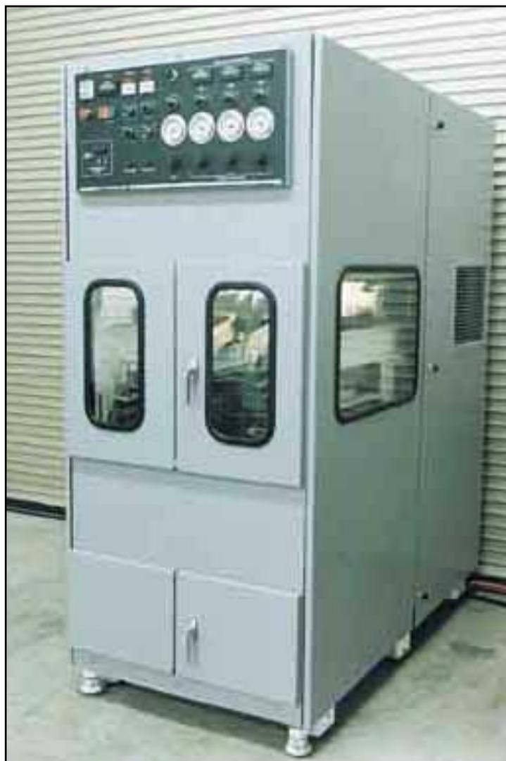
*The Asphalt Pavement Analyzer is a multi-functional loaded-wheel tester that has been successfully used for evaluating rutting, fatigue cracking, and moisture susceptibility of both hot and cold asphalt mixes.*
