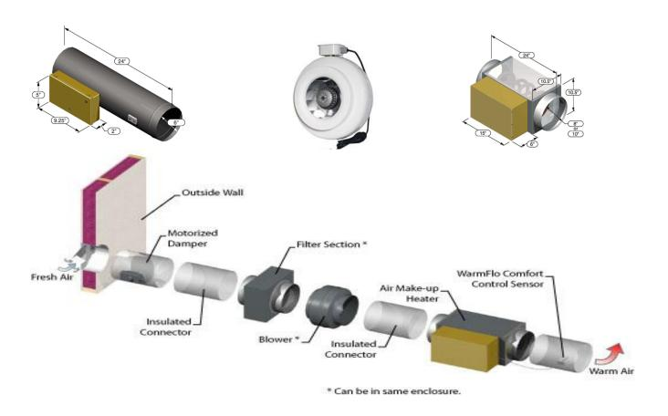
These units provide tempered fresh air for code requirements and/or appliances which could create unhealthy negative pressure within the building. <a href="http://www.electromn.com/gen/makeup\_air.htm">http://www.electromn.com/gen/makeup\_air.htm</a>
