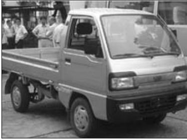
four-wheel Truck XL, a low-speed (25 mph) vehicle with 800 lb payload for industrial and utility fleet purposes, to
