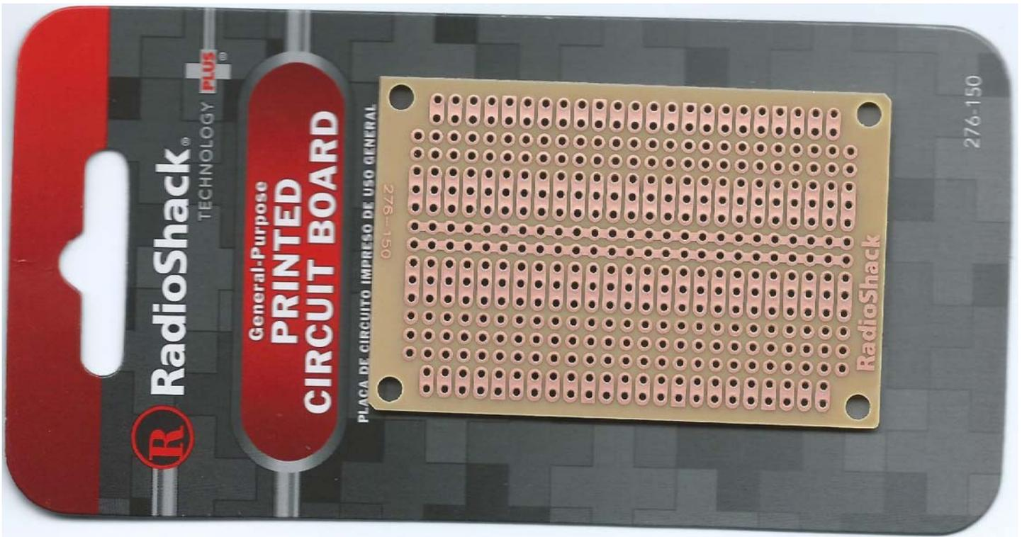
I found the first one at Radio Shack for about \$3. The Shack had other sizes and even some round boards, but this one has holes spaced the closest together.
