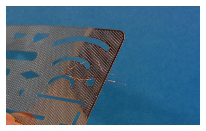
I inserted both ends of a length of thin wire in two holes that are spaced apart the distance I need.
