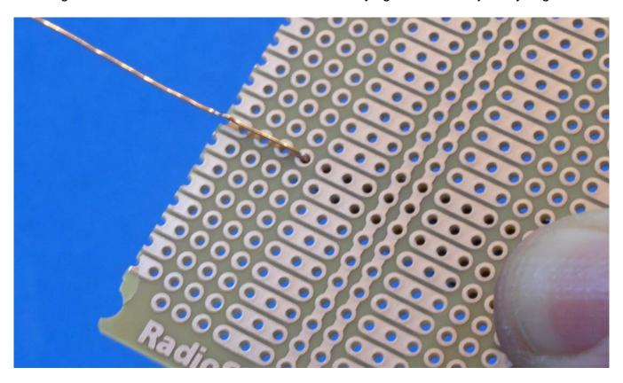
Next I bent the wire across the board, pulling it tight to make the first 90 degree bend.
