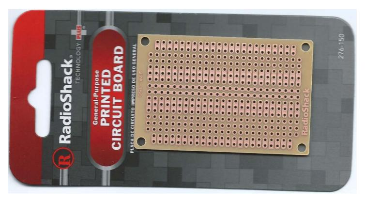
I found the first one at Radio Shack for about \$3. The Shack had other sizes and even some round boards, but this one has holes spaced the closest together.
