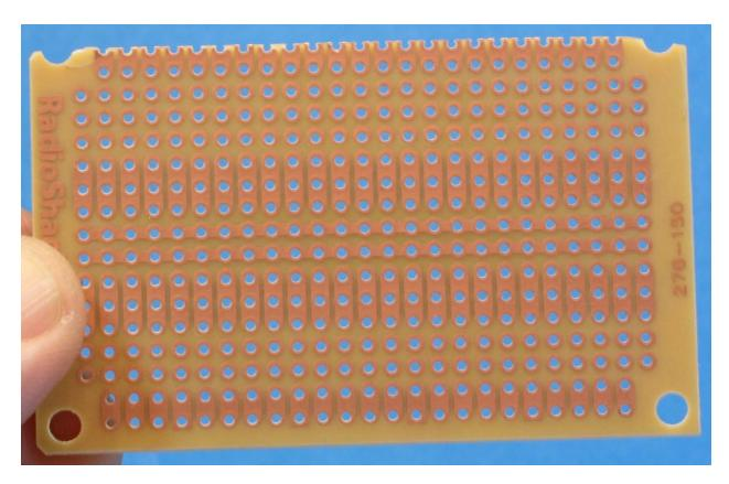
I sanded/filed one of the long side edges until the edge runs through the center of the outside set of holes. Note – sand/file towards the face of the board with the copper printing, otherwise they probably will be pulled away from the board. The sanded edge created "notches" that should make it easier to make the second bend in the wire.
