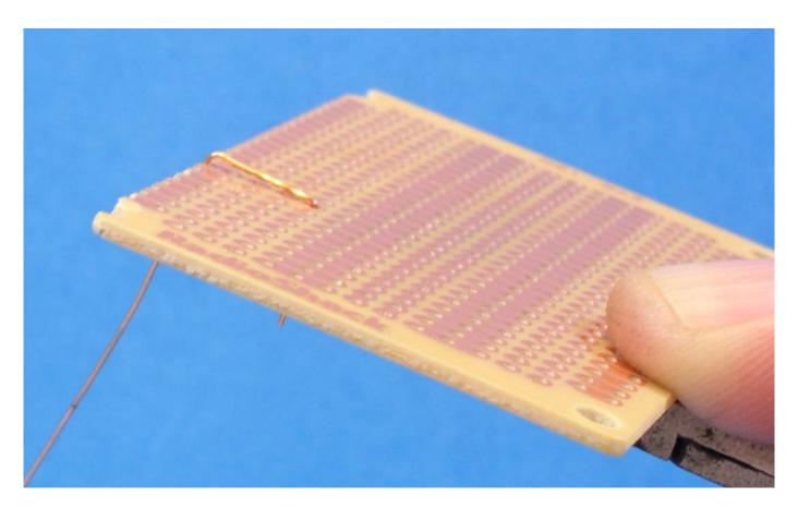
I bent the wire into an edge notch to make the second 90 degree bend, pulling it tight to make a tight bend.
