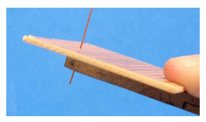
For bending a grab handle, I insert one end of the wire into a hole and hold the end with a pair of pliers flat against the underside. This is more secure than trying to do so with just my fingers.
