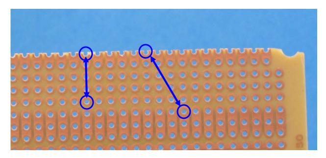
I'll measure which hole to a "notch" is close enough to the size I need. The appropriate hole and notch may be horizontal on the same row, or may be diagonally on different rows. Also, the hole and the notch could be marked with a colored marker.
