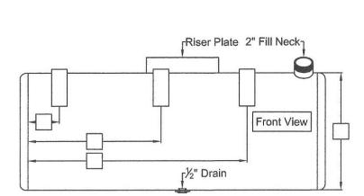
Please note: All sizes are NPTF unless otherwise noted and reference all measurements from the lateral weld seam and the end cap weld seam to the center of the fittings.
