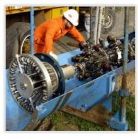
ILI tools identify pipeline sections belonging to same manufacturing batch.
