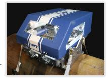
MMT's HSD Tester is used in-ditch at each batch location to verify material strength.
