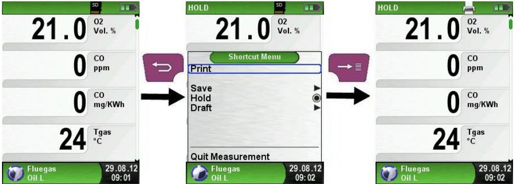
Fig 6: Direct access menu, (ex.: Flue gas measuring)
