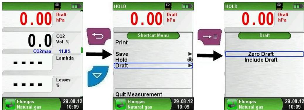
The measured draft is displayed continuously in the main display (red coloured). After the confirmation of the draft value with "Include Draft" the value will be included in the record and will be displayed in black colour.
