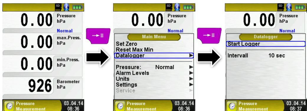
Start the Data Logger with the “Enter” button on “Start Logger”. In the lower field of information the time progress of the logger is shown.
