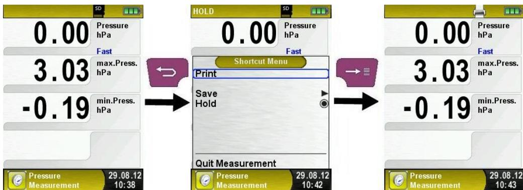
As soon as the print command is chosen, the record is printed parallel to the measuring task (→multitasking function), i.e. the measurement mode remains active.
