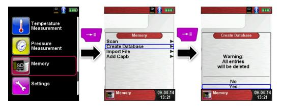
With this procedure a file named DATABASE.CSV will be generated on the MicroSD card. This file will show the database entries of the BLUELYZER<sup>®</sup> ST. This process needs a few seconds.
