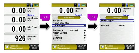
Start the Data Logger with the "Enter" button on "Start Logger". In the lower field of information the time progress of the logger is shown.
