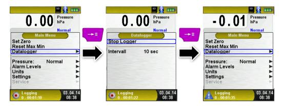
The logged values will be stored on the MicroSD card in the folder "LOGGER\Date. File name is the starting time. Every 7200 lines the device will automatically create a new XLM log file. With a logger interval of 1 second and a 1 GB MicroSD card it is possible to log in minimum a time period of 2 months.
