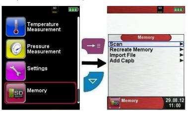
Before the first use of a MicroSD card, the memory structure should be created.
