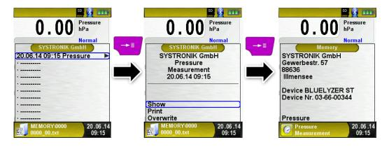
The customer information will be shown in the header of the measurement report. The saved file can be opened with a web browser (e.g.: Chrome, Firefox, Explorer, Opera, etc.)
