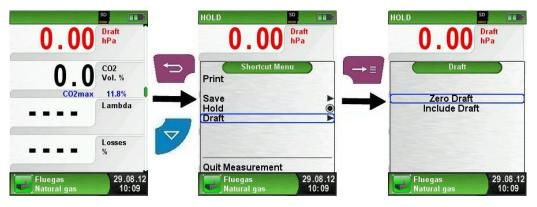
The measured draft is displayed continuously in the main display (red coloured). After the confirmation of the draft value with "Include Draft" the value will be included in the record and will be displayed in black colour.
