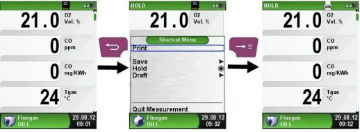
Fig 6: Direct access menu, (ex.: Flue gas measuring)
