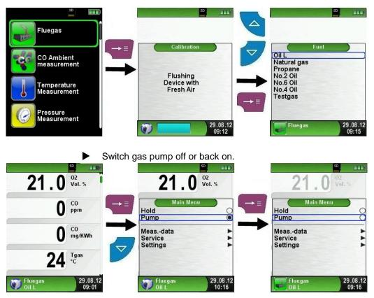
When the gas pump is switched off, the pump symbol is no longer shown in the status bar. Changes in the corresponding measured gas values cannot be ruled out, e.g. the O2 value may change as a result of lack of oxygen in the gas lines inside the device. If the gas pump remains off for a longer period of time, calibration in fresh air should be carried out before a new measurement is made.
