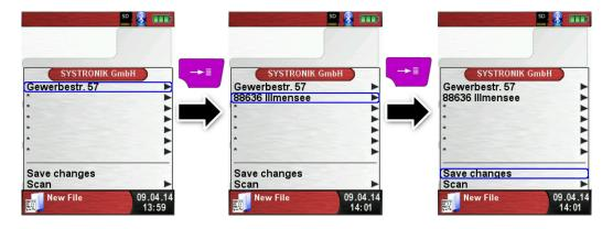
To delete customers in the database there mustn't be any measurements stored. Select the customer and choose "Scan", if there are no measurements stored the request "Entry is empty delete?" will occur. Confirm the request with "Yes".
