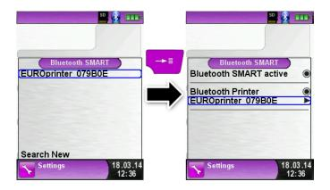
The IR modus could be set by deactivating the "Bluetooth Printer" in the settings menu. Set the printer to IR modus as well. Press the keys "OFF" and "ON" at once and the blue flashing LED goes out.
