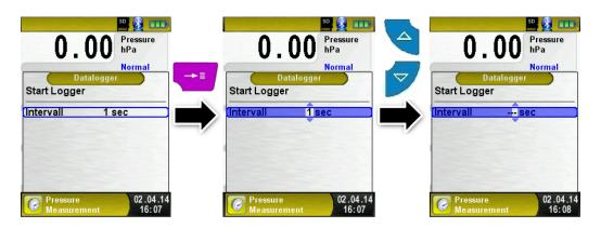
Than confirm with the "Enter" button and set the second number. Again confirm with "Enter" button and finally set the third number. Confirm the number with "Enter" button.
