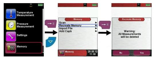
The memory structure consists of 100 memory locations, which can be described in each case with a measuring protocol.
