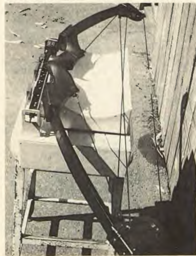
A closeup of the bow scales shows the holding weight of the Golden Comanche at twenty-nine inches.
