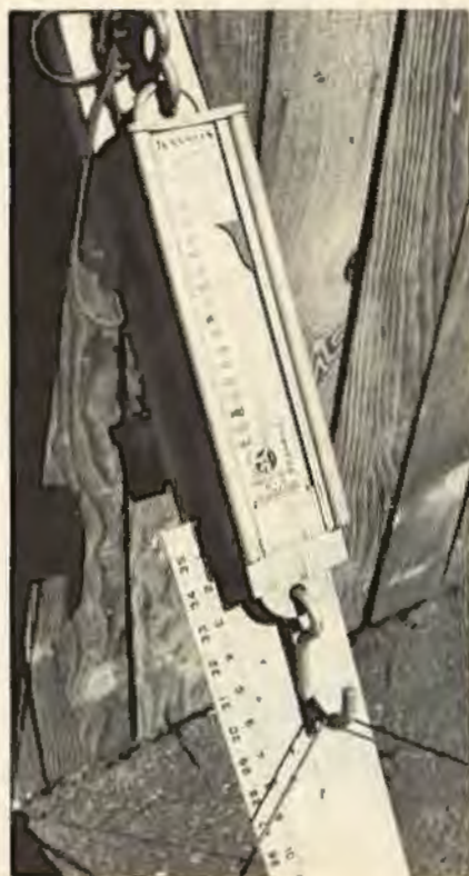
A closeup of the bow scales shows the holding weight of the Golden Comanche at twenty-nine inches.
