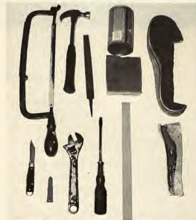
You need a hacksaw, center punch, jackknife, file, screwdriver, crescent wrench, shoe portion, can, foam piece, aluminum bar and bench vise (not shown).
