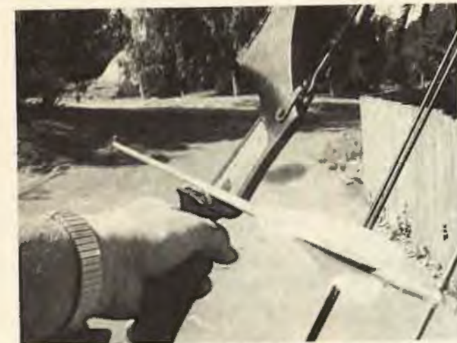
This side view of an arrow on the cable shows that there is no rippling of the fletching — which often occurs when there is cable involvement.
