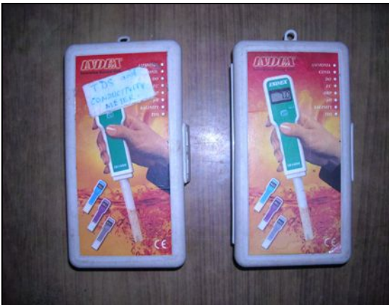
Fig. 5.2. INDEX model pH, TDS and conductivity test kits.
