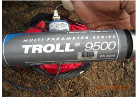
Fig. 5.1. YSI (Yellow Spring Instrument) multipurpose model no. 6600 and TROLL multi-parameter series no. 9500.
