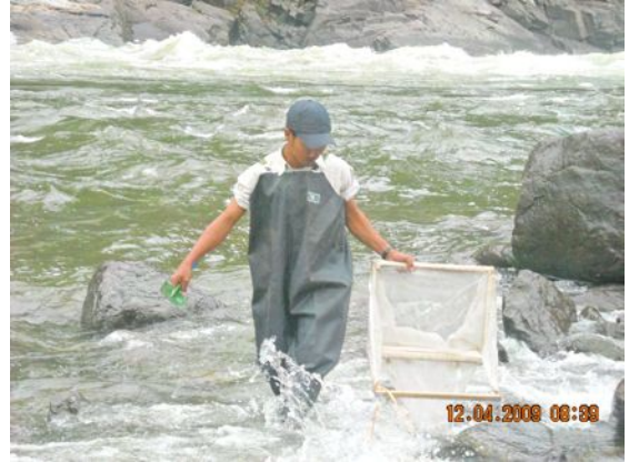
Fig 5.6. Benthos sampling using D-shape kick-net.
