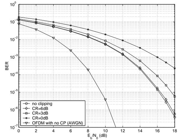
Fig. 8. BER versus  $E_b/N_0$  in a multipath channel for varying CR values.
