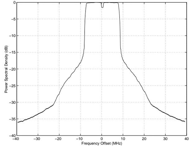
Fig. 2. Power spectra of the clipped HIPERLAN2 OFDM signal. CR = 2.0 dB.
