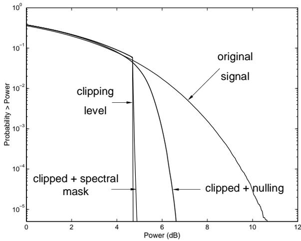
Fig. 5. CCDF for OFDM signals after clipping and spectral masking. CR = 4.5 dB.
