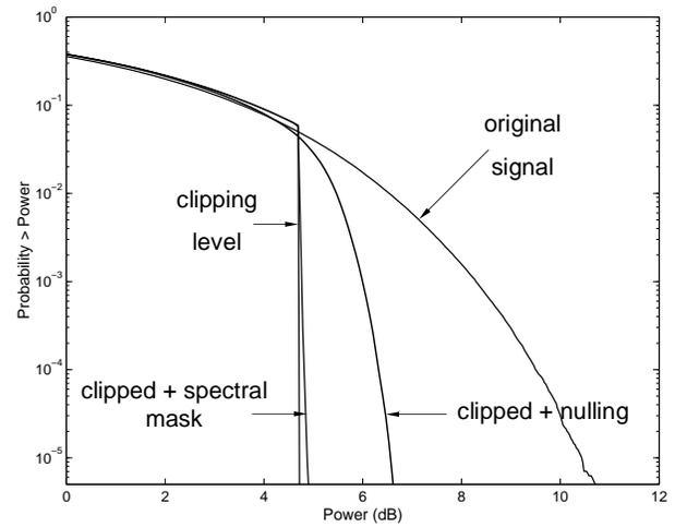
Fig. 7. CCDF for OFDM signals after clipping and spectral masking (3 dB below the HIPERLAN2 mask). CR = 4.5 dB.
