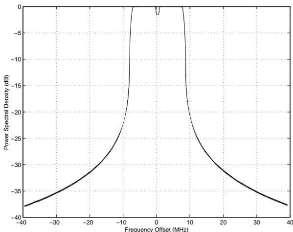
Fig. 1. Power spectral density of the HIPERLAN2 OFDM signal.
