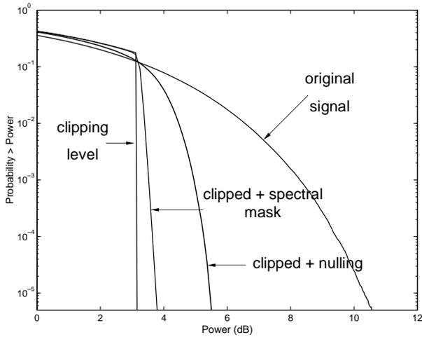
Fig. 6. CCDF for OFDM signals after clipping and spectral masking. CR = 2.5 dB.
