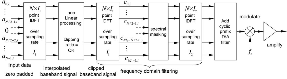
Fig. 3. Block diagram of the spectral masking PAPR reduced OFDM system.
