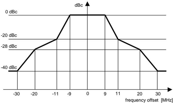
Fig. 4. Spectral power mask of OFDM based HIPERLAN2.
