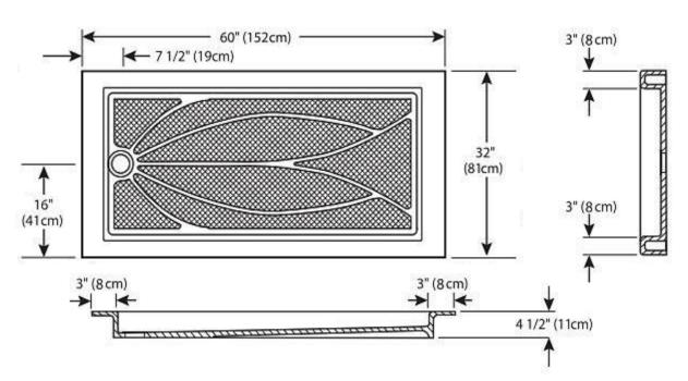
NOTE: In the casting process slight shrinkage in lenght will occur 1/8 "- ½"
