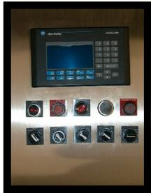
*Operator control stations range from Local pushbutton stations to panel mounted displays/terminals.*
