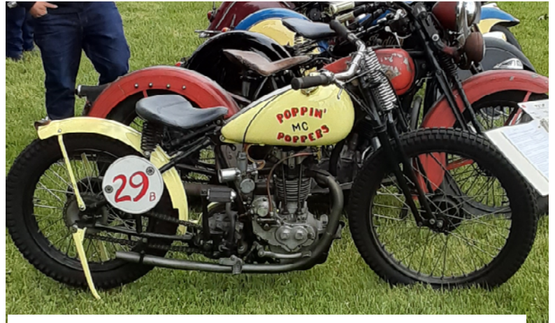
Martin Doerfler's 1928 Harley Model B with a 21 ci with overhead valve top end.
