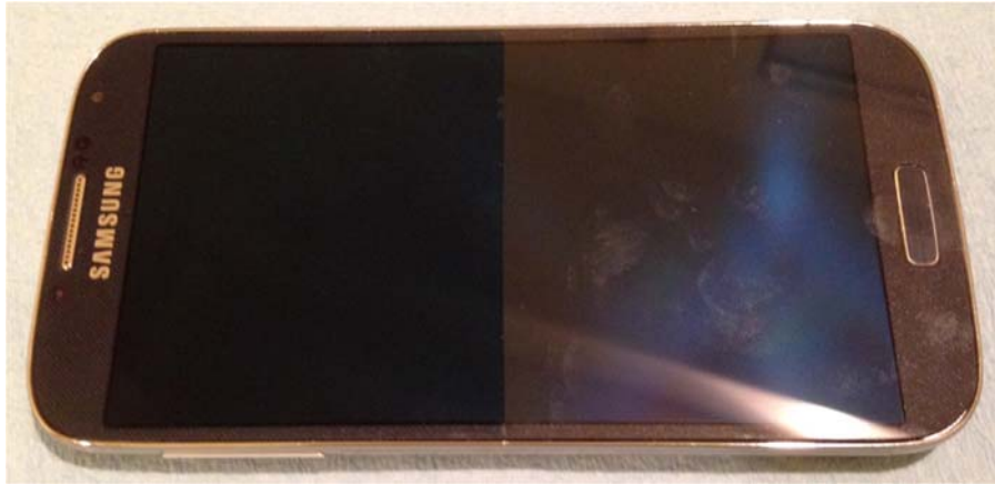
Figure 6: Anti-Fingerprint demonstration shows top side AR+DLC resists fingerprinting (top half coated with AR+DLC)
