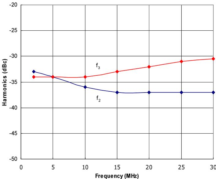
Figure 3: RFPS2-30-25 Typical f<sub>2</sub> and f<sub>3</sub> @ P<sub>out</sub> = 25W.
