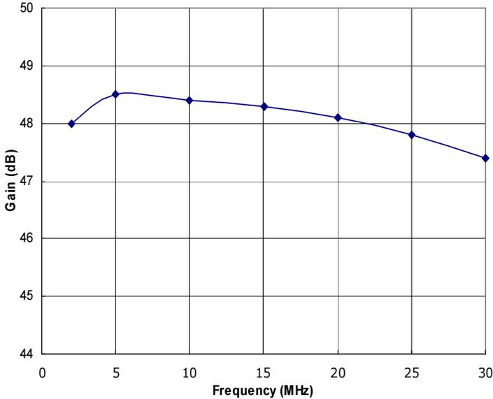
Figure 1: RFPS2-30-25 Typical Gain @ P<sub>out</sub> = 25W.
