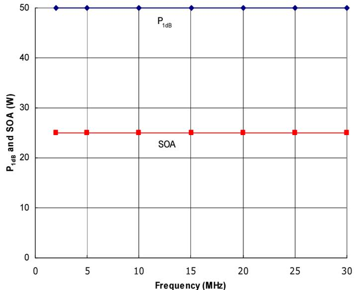
Figure 4: RFPS2-30-25 Typical P<sub>1dB</sub> and Safe Operating Area (SOA). The amplifier is capable of delivering much more power than it is safe to generate. Do not exceed the SOA shown above.
