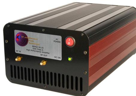
The RFPS2-30-25 is a Class A high performance amplifier mini-system, complete with power supply, heatsink, fan and thermal protection. It is excellent as a standalone military communications system driver, or as a driver for production testing or broadband systems development. It exhibits superior full power and back-off linearity, and utilizes a combination of two device technologies for optimum performance and ruggedness.
