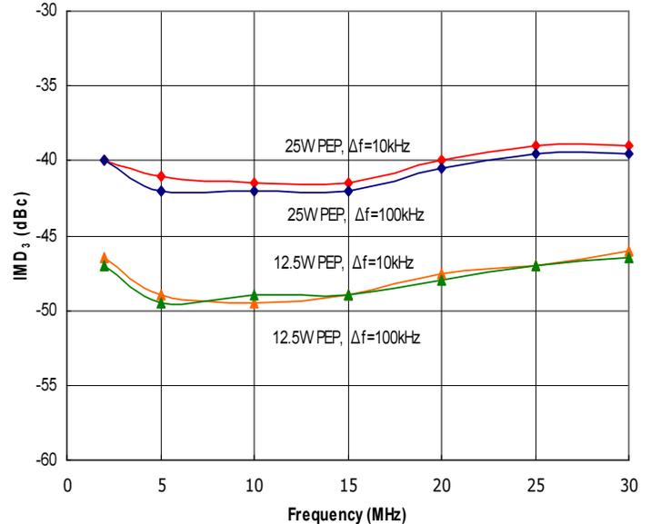
Figure 2: RFPS2-30-25 Typical IMD<sub>3</sub>, @ 25W and 12.5W PEP, Δf=10kHz and Δf=100kHz.
