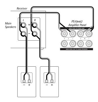
**Option 3**Connect the amplifier to the main speaker system and the main speaker system to the subwoofer in.
