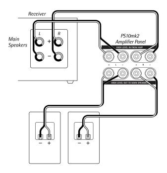
**Option 2**Connect both the subwoofer and the main speakers to the back of the receiver.
