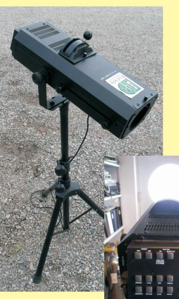
DMX Connectors: 3-pin Colors: 7 + white Gobo Size: 23.7mm outside, 21.3mm image, 1mm Light Source: 1 (white) 75W (18A) LED 50,000hrs Strobe Rate: 0 - 16Hz Stand Height: 2.8 - 3.8ft (0.8 - 1.2m) Zoom Angle: 14° - 20° Iris (min): 5° (at tightest zoom) Illuminance: 8,140 lux @ 2m (14°) Illuminance: 4,650 lux @ 2m (20°) Color Temperature Range: 6,500 7,500K Fits Tripod Sizes: 1.25in (33mm) Input Voltage: Switchable 120/230VAC 50/60Hz Power and Current: 215W, 1.8A @ 120V 60Hz Weight: 13.3lbs (6kg)
