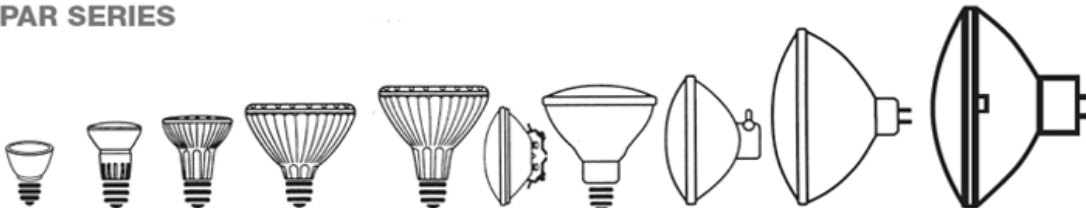
PAR14 PAR16 PAR20 PAR30 Short Neck PAR30 Long Neck PAR36 PAR38 PAR46 PAR56 PAR64
