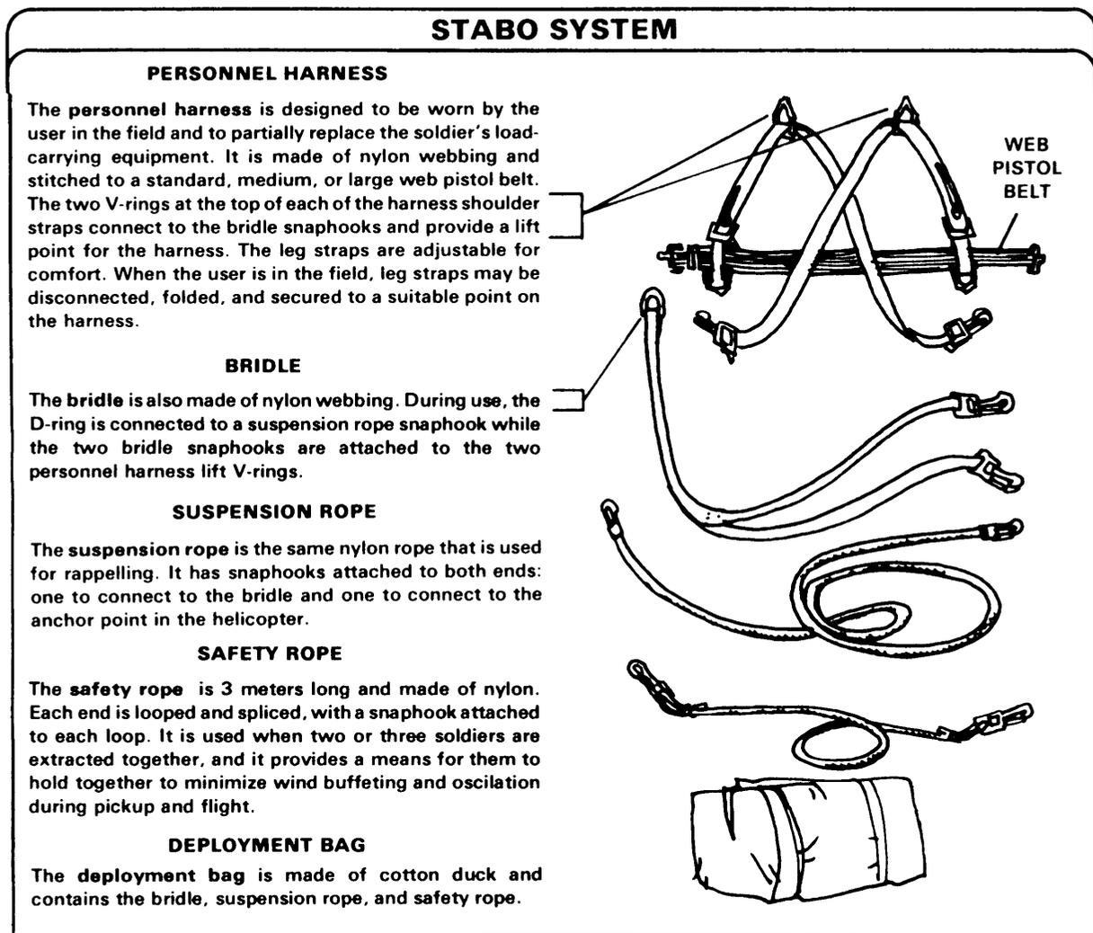
altitudes up to 150 feet. A member of the helicopter crew drops the extraction system deployment bag from the left door of the helicopter. (A maximum of three units may be connected and dropped simultaneously.) As the deployment bag descends, the suspension rope deploys until the bag reaches the ground. The soldier to be extracted then attaches the bridle snaphooks to the lift V-rings on his harness. After insuring that the leg straps are connected
