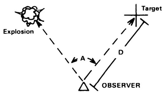
To calculate the correction in deviation, multiply angle A by distance D, with the distance expressed in kilometers, as shown in the example.
