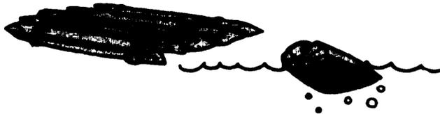
Logs, either singly or lashed together, can be used to float soldiers and equipment. Be careful when selecting logs for rafts. Some jungle trees will not float. To see whether certain wood is suitable, put a wood chip from a tree in the water. If the chip sinks, so will a raft made of that wood.
