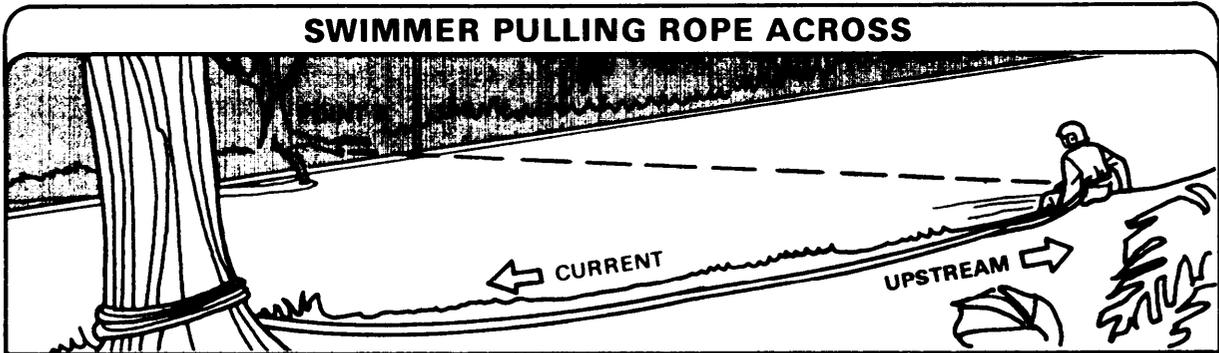
**One-Rope Bridge.** A one-rope bridge can be constructed either above water level or at water level. The leader must decide which to
