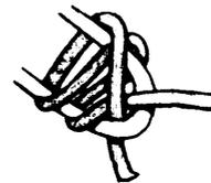
The double sheet bend knot is used to tie ropes of unequal diameter together.
