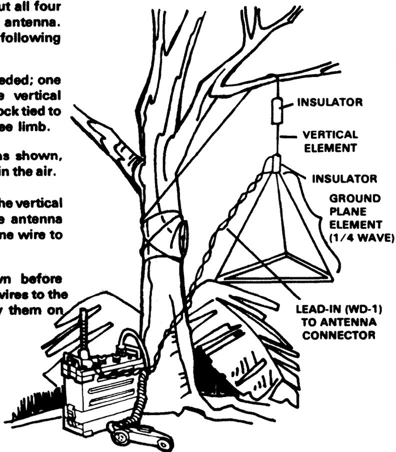
A third type of expedient antenna used in the jungle is the *patrol antenna*. It is the same as the jungle antenna minus the ground plane element. Insure that the length is determined by using the  $1/2$  wavelength instead of the  $1/4$  wavelength column of the chart. The range of the set will be increased 2 to 3 times its normal range. This antenna is easier to handle and construct.
