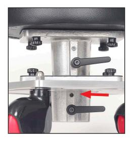
\* Note: It is necessary to temporarily remove the lower Kipp handle from the Base Flange in order for it to fit through the bottom of the Sneaker Base. (see red arrow) Only 1 Kipp handle is used in the Base Flange when installed inverted.
