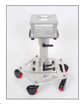
Important Note: It is not recommonded to setup higher than shoulder level in this configuration. Clearly, in this build, the center of gravity and mass of the camera sit high on a narrow base and can tip over if not careful. For this reason it's highly advisable that whenever built in high Mitchell Mode, someone remain close to the camera at all times and common sense is exercised.
