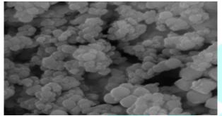
Figure 3. SEM image of synthesized zinc oxide nanoparticles
