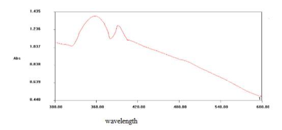
Figure 1. UV-Vis spectra of synthesized zinc oxide nanoparticles
