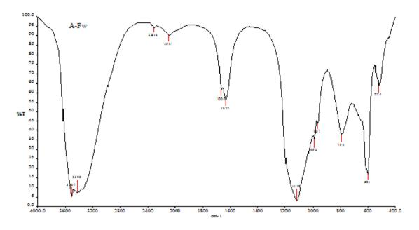
Figure 2. FT-IR spectra of synthesized zinc oxide nanoparticles
