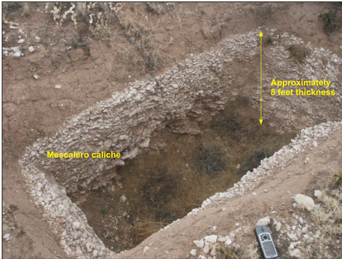
Figure 2.3.2.1-5 Photo of Mescalero Caliche in Test Pit South of the Pronghorn Saltwater Disposal Inc Facility
