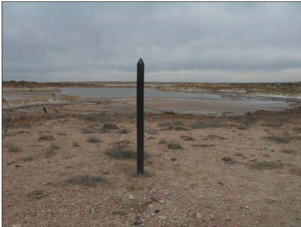
Figure 2.3.4.2-3 Well monument near Laguna Gatuna showing no signs of tilting or displacement
