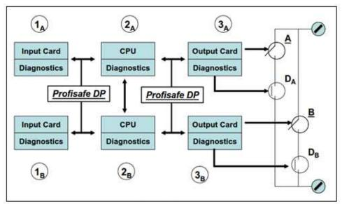
Figure 5-2: Example architecture SIMATIC S7-400FH
