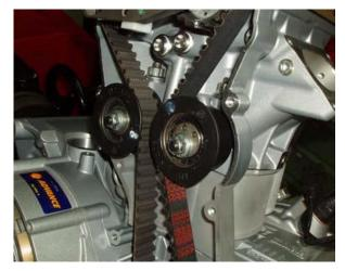
Install the belts, vertical cylinder first: bottom pulley first and work your way up.
