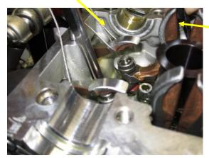
Block the oil return holes to prevent the retaining rings from falling into the cylinder.
