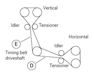
Set the belt frequency at 110HZ for all 4-cam engines. Measure at points D and E to get an accurate frequency measurement.
