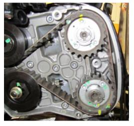
Additional notes on setting the engine to "home" and/or TDC in general. At TDC the arm on the turning tool will point towards the spark plug of the cylinder at TDC.
