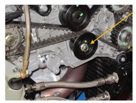
Loosen the tensioning pulley loosening the Fuji nut and rotating the tensioning pulley clockwise (away from the cam drive gears). Loosen the nut and remove the tensioning pulley from its mounting stud on the cylinder head. Removing the tensioning pulley facilitates belt removal/installation. Label the tensioning pulley (horizontal or vertical).
