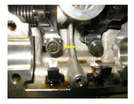
Here is the horizontal cylinder with the cams removed. You can see the opening shim has been removed from the valve on the left and the closing shim is accessible. The valve on the right still has the opening shim installed
