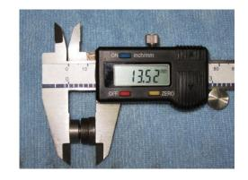
Add/subtract column [H] to column [I] to find: [J] the size of the closing shim to bring the clearance into specification. The closing shims can be sanded into the exact size with 400 wet/dry sandpaper if one of the standard sizes does not bring the clearance close enough to the desired measurement. Sand the closing shims on the "top" part of the shim: the wider part that contacts the closing rocker arm.
