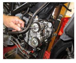
Use a punch and gently tap on the pulley to loosen the cam/cam retainers so the camshafts can be removed.
