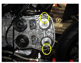
Align the marks on the cams with the engine cases for the vertical and horizontal cylinders.
