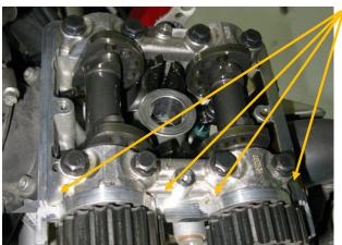
Put gasket sealant on the mating corners where the cam retainers meet the flat surface of the cylinder head/valve cover for sealing. Torque in two stages to 7ft lbs.
