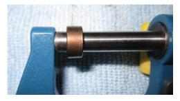
Close the micrometer. Do not over tighten. Press the "zero" button to set the reading to 0.00. Open the micrometer and place the shim on the stationary shaft of the micrometer, with the flat side towards the fixed portion of the micrometer. Measure the opening shim and record the measurement in column [D] of the worksheet. Determine the size of the replacement shim by adding/subtracting column [C] to column [D] and record this number in column [E].
