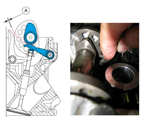
Use a feeler gauge (A), to measure the clearance between the opening rocker arm and the lower edge of the camshaft lobe: Use progressively larger/smaller feeler gauges until the size of the clearance can be determined. The proper feel is if the resistance on the feeler gauge is similar to inserting the gauge into a large book. Once the clearance is determined, record this as measurement [A] on the worksheet.
