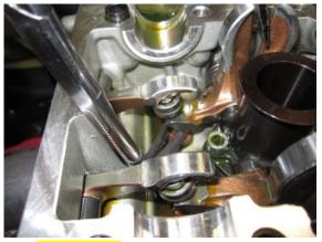
If a closing shim requires replacement, the opening shim will have to be removed from the valve. Remove the opening shim and set it aside, marking the shim's location for reassembly.
