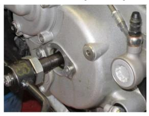
Remove the spark plugs. This is important: the engine will not rotate with the spark plugs installed. The engine is rotated during valve adjustment/belt replacement and rotation is made possible with the removal of the spark plugs and placing the transmission in neutral.
