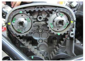
The torque stripes (green marks) do not necessarily indicate alignment.
