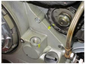
After the shims have been replaced (if required), install the camshafts. Apply oil or other lubricant to all mating (rotating) surfaces.
