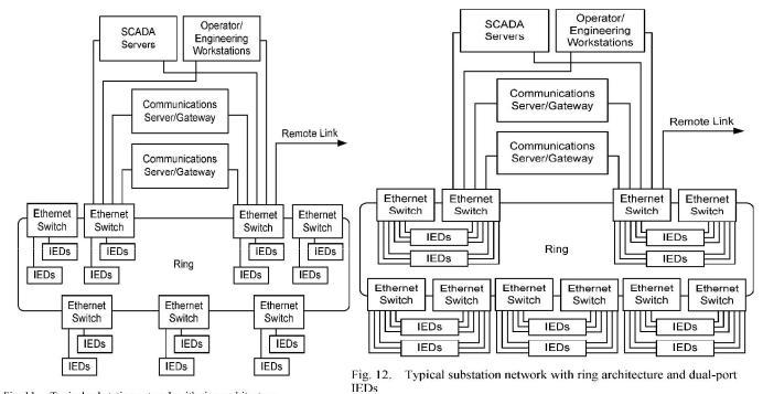
Fig. 11. Typical substation network with ring architecture
