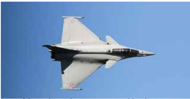
powerful punch. Twelve wing-mounted hard points can carry a combination of air-to-air missiles, air-to-ground missiles, sensors, and drop tanks. Despite the fact that the Rafale is now a 30-year-old design, upgrades such as the RBE2 AA active electronic scanning array (AESA) radar, Damocles targeting pod, Meteor air-to-air missiles, and SCALP cruise missiles have kept the design competitive
