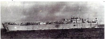
USS LST-16 underway in the Mediterranean area. Note the USAAF L-4 Grasshopper on the 220ft x 16ft flight deck ready for take-off.
