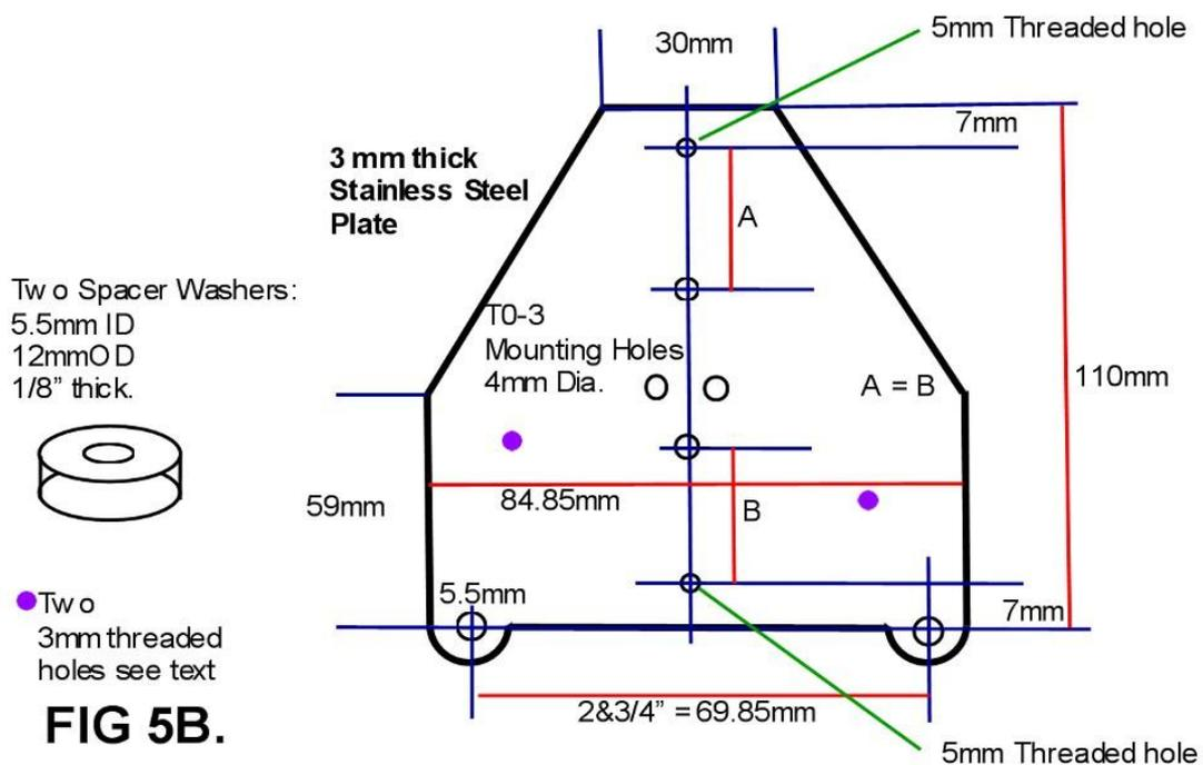
Ideally the screws are brass for low electrical resistivity. Brass 4BA screws are about the same diameter as 6-32 screws and are available from RS components, Newark or Element 14.
