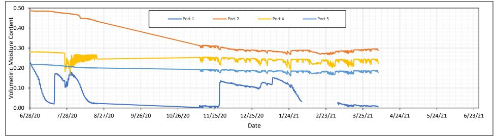
Figure 5. Landgrebe L1 soil moisture probes June 28, 2020 to April 6, 2021
