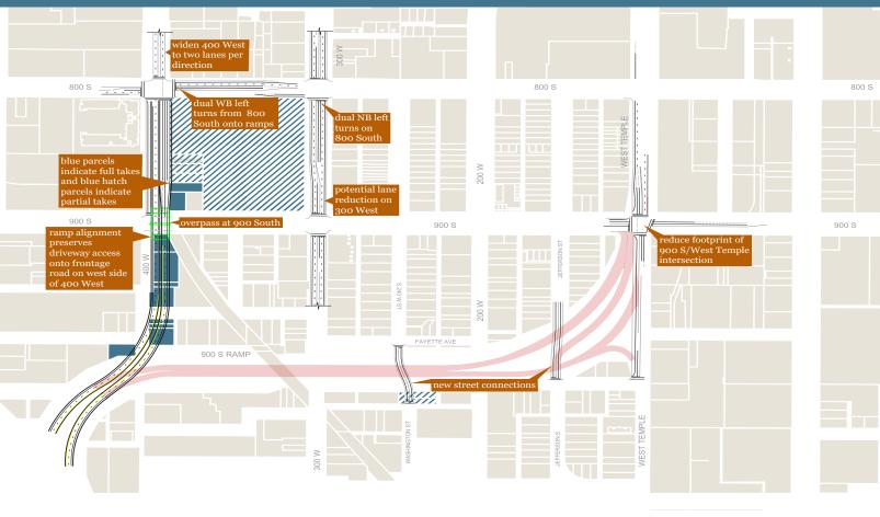
400 West: Realign ramps north along 400 West, passing over 900 South to touch down at 800 South
