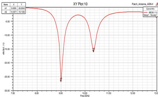
Fig.4: Return Loss ( $S_{11}$  parameters) Plot
