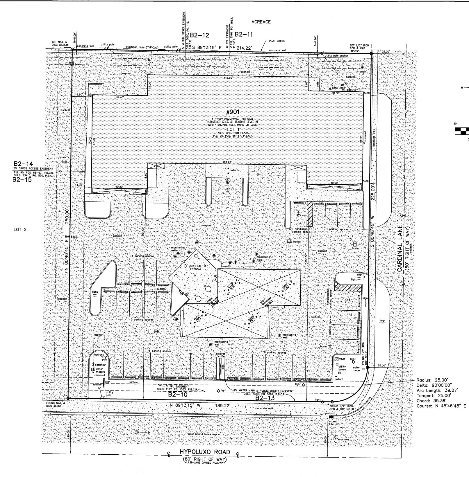
**LEGEND OF ABBREVIATIONS:** ELEVATIONS BASED ON N.G.V.D CENTRAL ANGLE SQUARE FEET PERMANENT CONTROL POINT P.C.P. = ARC LENGTH CHORD BEARING P.B.C.R. = RADIUS PLAT RIGHT OF WAY NAIL & DISC POINT OF CURVATURE P.O.C. POINT OF COMMENCEMENT P.O.B. POINT OF BEGINNING POINT OF TANGENCY AIR CONDITIONER WATER METER A/C OVERHANG FND. FOUND CHATTAHOOCHEE NORTH SOUTH F.P.L. FLORIDA POWER & LIGHT N.T.S. NOT TO SCALE EAST WEST B.C.R. BROWARD COUNTY RECORDS DADE COUNTY RECORDS
