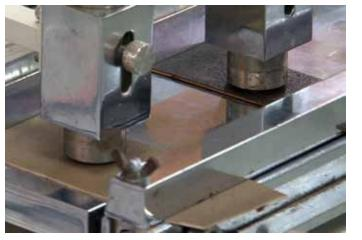
**MACHINES:** RUB TESTER **TEST EXAMPLES:** TEST THE COLOR FASTNESS TO-AND-FROM RUBBING OF LEATHER. PU. AND PVC.
