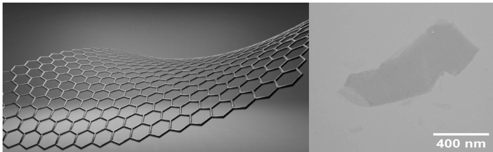
**Figure 1.** Graphene structure of 2-D fused aromatic systems and actual TEM image of isolated nanomaterial.
