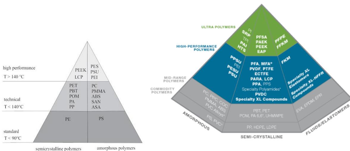
**Figure 1. Hierarchy of polymer materials and their stability (Tg and Tm) and possible degradation correlation. (images obtained from Ref. 2 and 3)**
