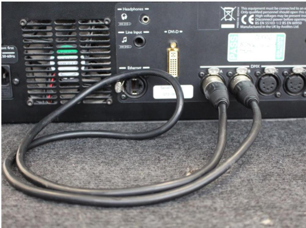
You will then need to shut down Titan using the tools menu in order to test the DMX ports.
