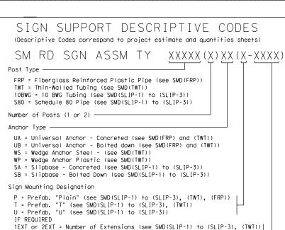
BM = Extruded Wind Beam (see SMD(SLIP-1) to (SLIP-3))
